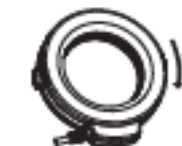
Installing a diffuser
